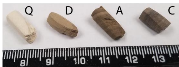
Figure S1. Example mini cores. Samples shown are quarry (opal-A), D 1341.1 (opal-A), A 1017.0 (opal-CT), and C X524.3 (diagenetic quartz). Letters indicate the sample source (quarry or field). Their assigned silica group is provided in parentheses. Scale is in cm. More information about the sample sources and silica groups are in Ross and Kovsky (2022).
