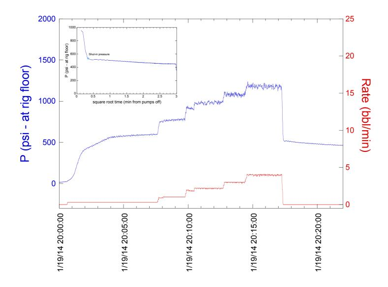
Figure S1: Stepped rate injection test (SRIT) record, showing pumping rate (red curve) and pressure measured at the rig floor (blue). Leak-off pressure (LOP) during initial injection is consistent with the interpreted shut-in pressure after pumps were turned off.
