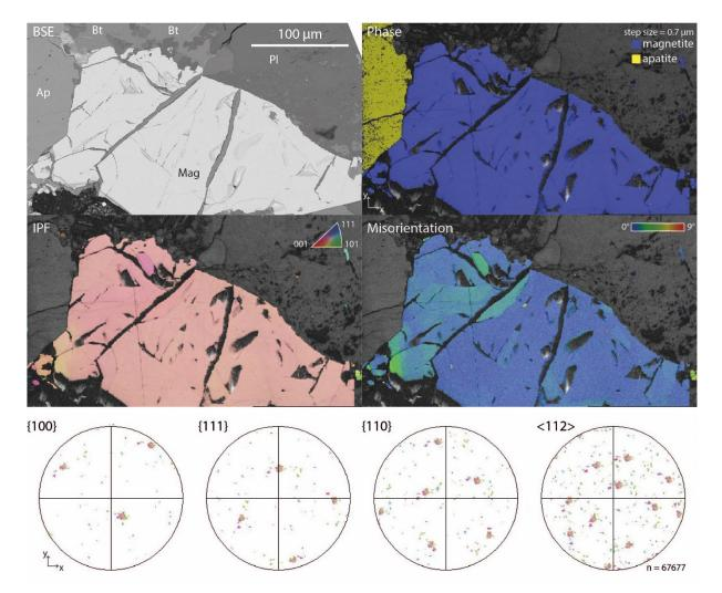
**Item S3B.** EBSD data for sample 5, grain 2. From top left: BSE image with phases marked, phase information map + BC, IPF map denoting the grain orientation + BC, misorientation map + BC, and pole figures. Stereo net projections are equal area, lower hemisphere. BC = Band contrast; IPF = Inverse pole figure. Pl = plagioclase, Mag = magnetite, Hem = hematite.
