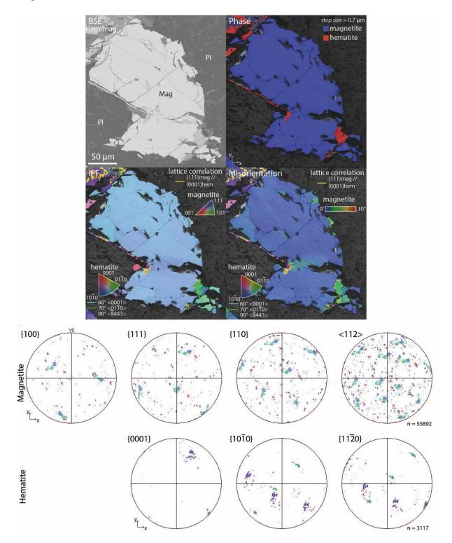
**Item S3C.** EBSD data for sample 5, grain 3. From top left: BSE image with phases marked, phase information map + BC, IPF map denoting the grain orientation(s) + BC, misorientation map + BC, and pole figures. Stereo net projections are equal area, lower hemisphere. BC = Band contrast; IPF = Inverse pole figure. Pl = plagioclase, Afs = K-feldspar, Bt = biotite, Mag = magnetite.
