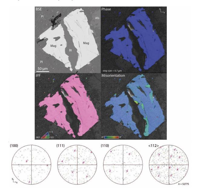
**Item S4A.** EBSD data for sample 21, grain 1. From top left: BSE image with phases marked, phase information map + BC, IPF map denoting the grain orientation(s) + BC, misorientation map + BC, and pole figures. Stereo net projections are equal area, lower hemisphere. BC = Band contrast; IPF = Inverse pole figure. Pl = plagioclase, Bt = biotite, Qz = quartz, Mag = magnetite, Ap = apatite.
