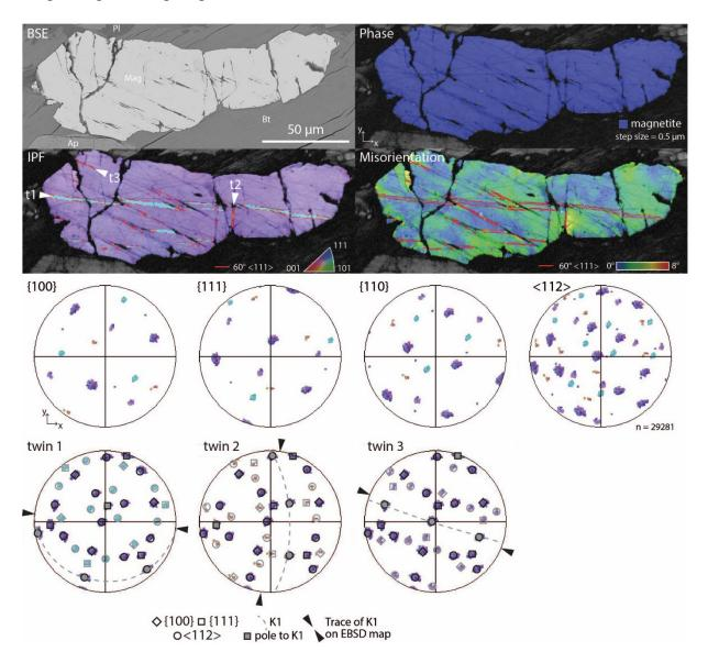
**Item S6D.** EBSD data for sample 69, grain 4. From top left: BSE image with phases marked, phase information map + BC, misorientation map + BC, IPF map denoting the grain orientation(s) + BC, and pole figures. Stereo net projections are equal area, lower hemisphere. BC = Band contrast; IPF = Inverse pole figure. Qz = quartz, Bt = biotite, Mag = magnetite, Ap = apatite, Ttn = titanite.
