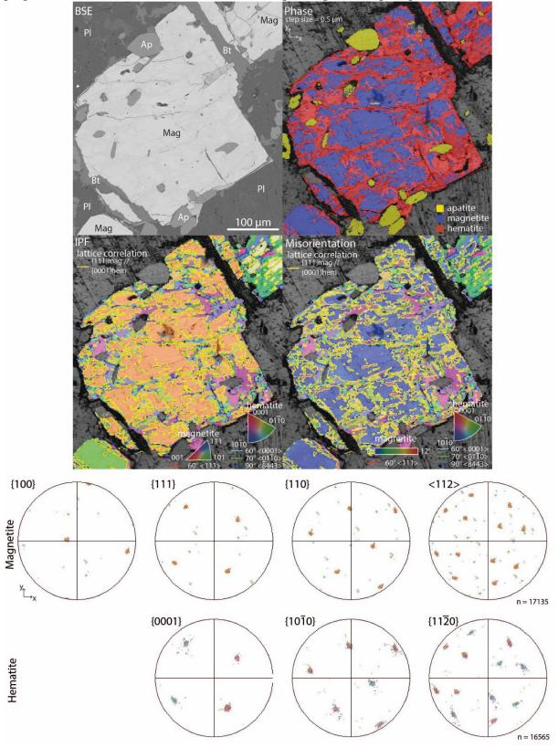
**Item S5B.** EBSD data for sample 58, grain 2. From top left: BSE image with phases marked, phase information map + BC, IPF map denoting the grain orientation + BC, misorientation map + BC, and pole figures. Stereo net projections are equal area, lower hemisphere. BC = Band contrast; IPF = Inverse pole figure. Pl = plagioclase, Bt = biotite, Mag = magnetite, Ap = apatite.
