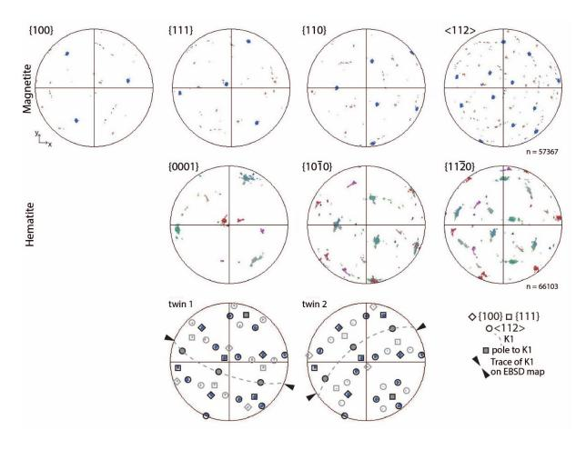
**Item S4B.** EBSD data for sample 21, grain 2. From top left: BSE image with phases marked, phase information map + BC, IPF map denoting the grain orientation + BC, misorientation map + BC, and pole figures. Stereo net projections are equal area, lower hemisphere. BC = Band contrast; IPF = Inverse pole figure. Bt = biotite, Mag = magnetite, Ttn = titanite, Ap = apatite.
