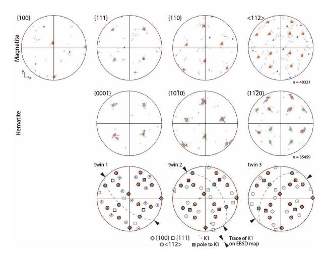
**Item S4C.** EBSD data for sample 21, grain 3. From top left: BSE image with phases marked, phase information map + BC, IPF map denoting the grain orientation + BC, misorientation map + BC, and pole figures. Stereo net projections are equal area, lower hemisphere. BC = Band contrast; IPF = Inverse pole figure. Pl = plagioclase, Bt = biotite, Hbl = hornblende, Mag = magnetite.
