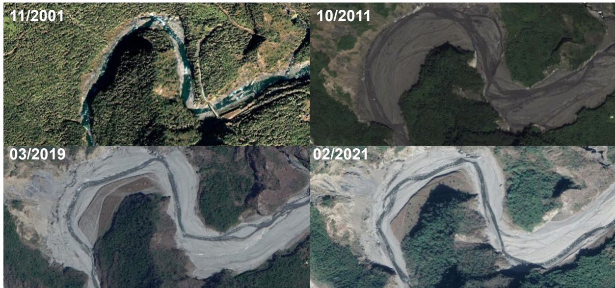
Figure S11. Example of time evolution of Morakot aggradation surface. Sediment is deposited during the 2009 typhoon Morakot. By 2019 a fill terrace has been abandoned, but the latest imagery shows that this surface is rapidly retreating and is likely to all be mobilized. Located in the Ailiao river (basin W9) at 267718m E, 2519189m N. UTM 51Q.
