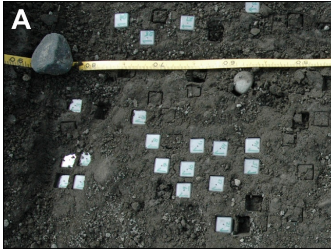
Figure DR2. Plastic boxes for AMS sampling inserted in a horizontal platform excavated in a flute. Owing to stones in till that commonly prevented boxes from penetrating, sampling grids tended to be irregular, as shown. (B) Boxes after having their orientations marked in situ and after their excavation and capping.
