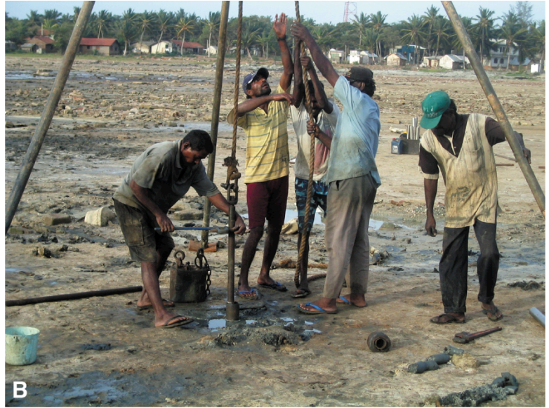
Figure DR4. Field photographs of Soil Tech, Ltd. coring in August 2005. The cores were collected using a weighted tripod system with a mixture of steel and PVC casings.
