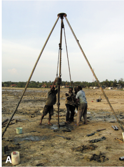
Figure DR4. Field photographs of Soil Tech, Ltd. coring in August 2005. The cores were collected using a weighted tripod system with a mixture of steel and PVC casings.
