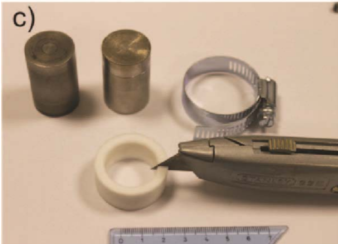
Figure DR9. (a) Disassembled components of the sample assembly used during the experiments; (b) Assembled stainless steel cylinders. (c) A Teflon ring is cut and then tightened to the stainless steel cylinders by a hose clip to confine gouges during the experiments. (d) Sample assembly in its fully assembled configuration.
