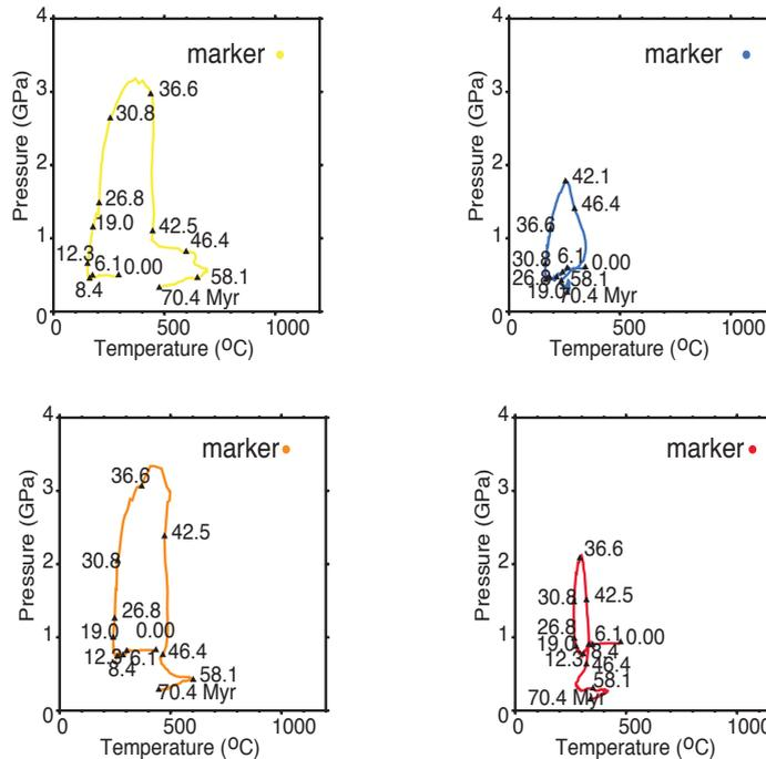
Supplementary Figure ÖÜ3: a) Final structure of the experiment with the position of the colored markers also presented in Supplementary Figure 2, b) pressure-temperature paths through time of the markers of block 1, c) pressure-temperature paths through time of the markers of block 2.
