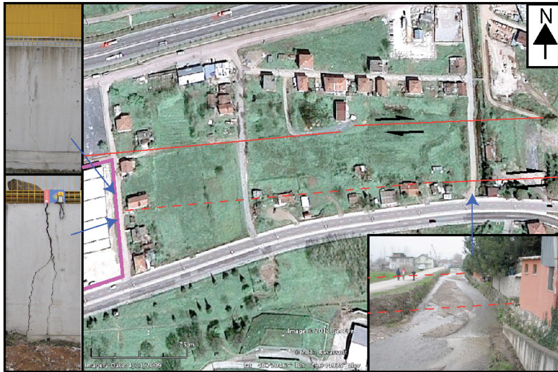
Figure DR1. Google Earth image (© 2011 Google, GeoEye, Başarsoft) and field photographs showing a deformed concrete wall (purple lines) built across the 1999 Izmit surface rupture zone (left panel) and a channel offset during the 1999 event (lower right panel) immediately south of Izmit. Red lines show coseismic fault trace.
