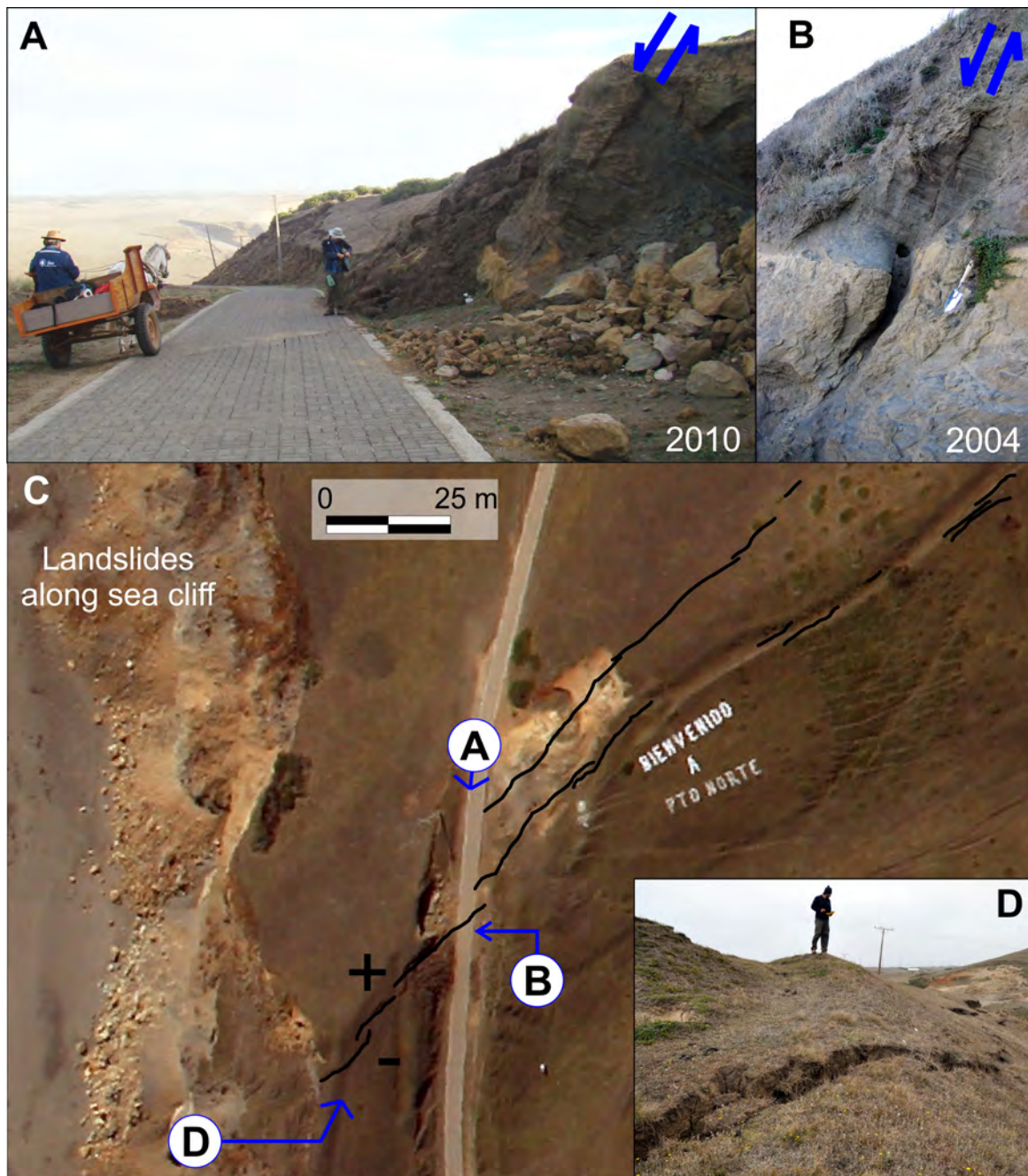
Figure DR6. Views of the western fault segment. A: Fault rupture across the paving stone with 15 cm of vertical throw and exposed on adjacent road cut; photo taken March 22, 2010. B: Same road cut photographed in March 2004, exposing a steeply-dipping fault with 15 cm of displacement, offsetting ~27-ka-old eolian strata. C: Vertical air photo (25-cm digital image from March 25, 2010) showing fault traces and location of field views. Signs indicate relative displacements. Note the presence of fresh landslides along the sea cliff, which covered fault exposures showed in Figure DR5. Note the label “Bienvenido a Pto Norte” east of the road, meaning “welcome to the town of Puerto Norte”. D: Close-up view of en échelon surface ruptures at the southwestern tip of this segment. Photo taken March 12, 2010, person for scale.
