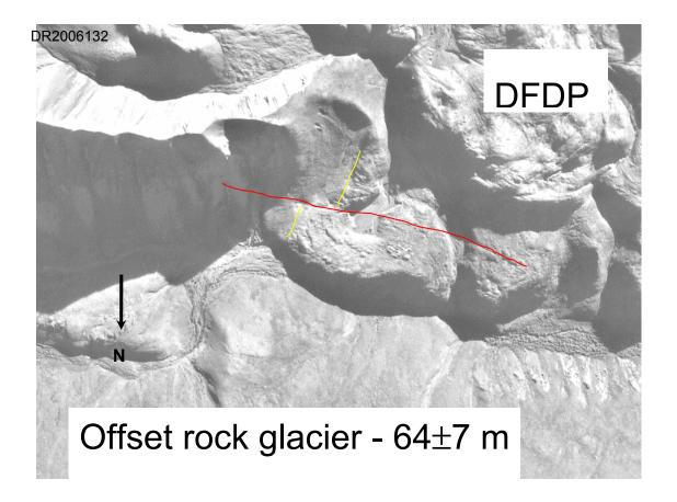
Offset was determined by the measured displacement of the eastern boundary (yellow lines) of this inactive rock glacier. Error expresses the uncertainty in determining the piercing point. Offset was measured with a measuring tape.
