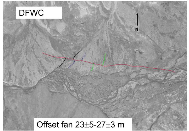
Alluvial fan – offset is measured by correlating eastern edge of the fan (green line), the western edge of the fan (black line) and a small channel within the fan (blue line). The uncertainty in the measurement is expressed both by the range of measured offsets and by the uncertainty on the location of each piercing point. Offset measurement was done by measuring tape.
