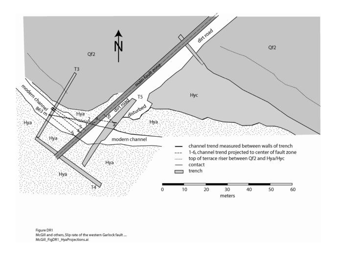
Figure DR1: Projection of late Holocene channel trends to fault. The letter "a" labels the trend of sub-channel "a" in trench 5 and its projection to the fault. The characters "863 m" mark the location and trend of the structure contour on the top of Qf1 in trench 3 that is at the elevation (863 meters) at which the base of sub-channel "a" in trench 5 is expected to project to the location of trench 3,
