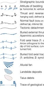
Stratigraphic boundary a b c d Attitude of bedding + / <sup>40</sup>/<sub>8</sub><sup>30</sup> (a: horizontal; b: vertical; c: upright; d: overturned) a b Thrust and reverse fault (triangles on the hanging wall); defined (a), inferred (b) a b Normal fault (ticks on the hanging wall); — Tectonic detachment Buried external thrust front of the Apenninic accretionary prism (C.N.R., 1983)
