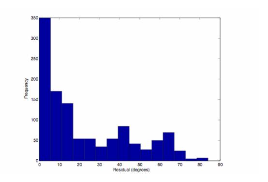
Appendix 3 Histogram showing total residual misfit of the "best fit" contemporary model with a median residual misfit value of ~12°. Modelled  $\sigma_H$  orientations were averaged over a small window whose centre corresponded to the location of a  $\sigma_H$  orientation with A to B quality for various regions over the Australian continent and continental margin. The difference between azimuths of measured and average modelled  $\sigma_H$  orientations then determined the residual misfit.
