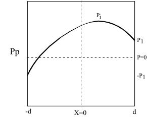
Using the two boundary conditions to solve for the two unknowns A and B, we get  $A = P_1/d$  and  $B = Wd^2/2K$ , where d is the half length of the specimen. This yields the pore pressure profile:
