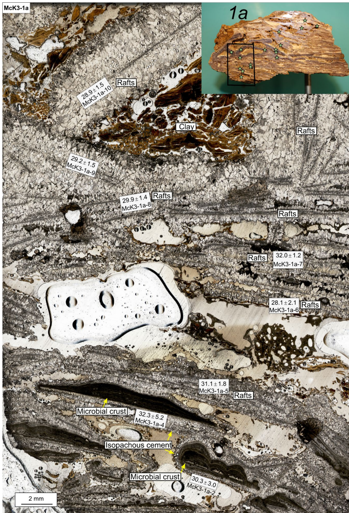
Fig. s7. Thin section of sample McK3-1a with location of U-Pb dated calcite stages (two isopachous cements; McK3-1a2 and 4; six rafts; McK3-1a5 to 10).
