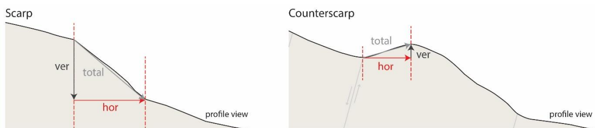
Figure S3: Schematic cross-section of how displacements were derived from scarp and counterscarp features along topographic profiles. The horizontal displacement estimate is based on the interpretation of changes in slope (indicated in red), and the vertical displacement is based on the resulting change in surface elevation (indicated in dark grey). The total surface displacement vector is indicated in light grey.
