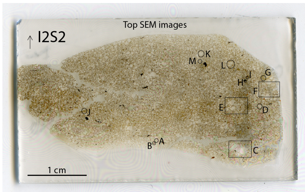
Figure S31: Scan of thin section I2S2, showing the locations analysed with SEM-EDS.
