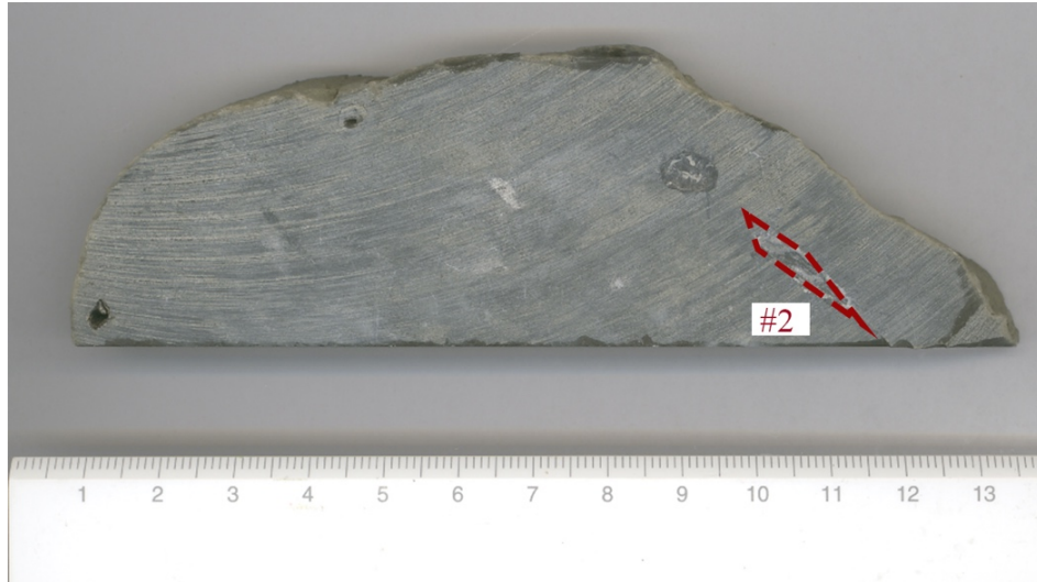
Figure S3. Scanned billet of methane derived authigenic carbonate AMNH loc. 3528 # 102525F (N-S). The area inside the red dash line is the region that was subsampled for clumped isotope measurement. Subsample #2 is an example of nodule (similar to the feature shown in Fig. S6a). Another subsample was taken right above #2, but it was not measured for clumped isotopes in this study. Details about the sample morphologies and isotopic results can be found in Table 1 and supporting data spreadsheet. Circular saw cut marks can be seen running across the samples surface. Scale units in this figure are in centimeters.
