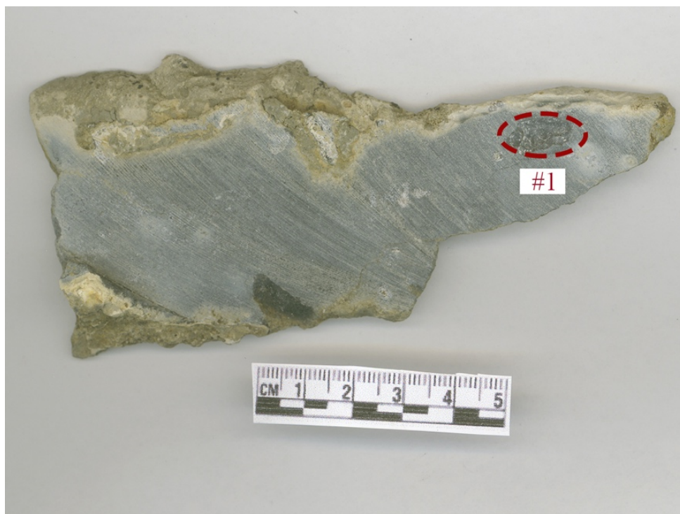
Figure S12. Scanned billet of methane derived authigenic carbonate AMNH loc. 3418 # 79159A. The area inside the red dash line is the region that was subsampled for clumped isotope measurement. Subsample #1 is micrite. The entire hand sample surrounded by notably lighter edges that were avoided during microdrilling. Details about the sample morphologies and isotopic results can be found in Table 1 and supporting data spreadsheet. Circular saw cut marks can be seen running across the samples surface.
