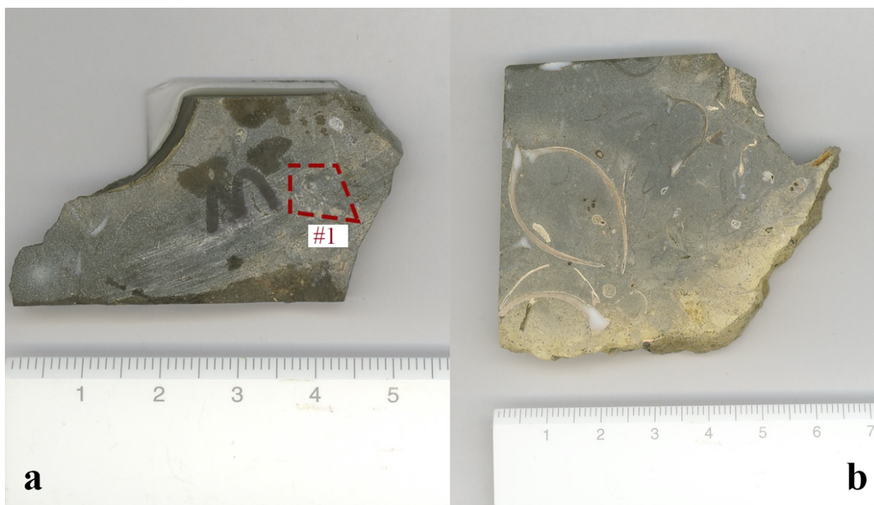
Figure S15. Scanned billets of methane derived authigenic carbonate AMNH loc. 3440 # 102535B. The area inside the red dash line is the region that was subsampled for clumped isotope measurement. #1 is an example of micritic coquinite. The scan in (b) is a more representative coquinite (with shell fragment embedded) from the same sample hand sample. Details about the sample morphologies and isotopic results can be found in Table 1 and supporting data spreadsheet. Scale units in this image are in centimeters. Some circular saw cut marks can be seen running across the sample surface in (a).
