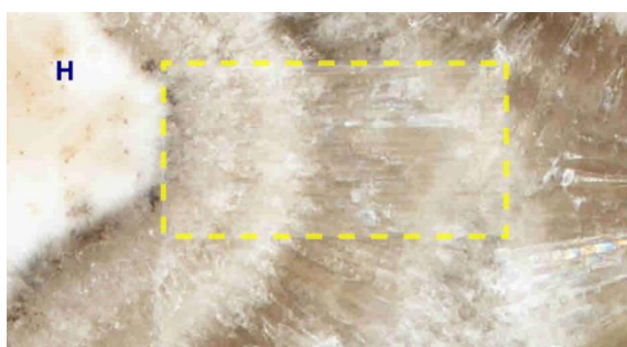
Figure S6 , image of polished block surface with botryoidal C_1 growing on host micrite (H). Area of C_1 chosen for elemental mapping indicated by yellow stippled box. The mapped area is 1 x 2 mm.
