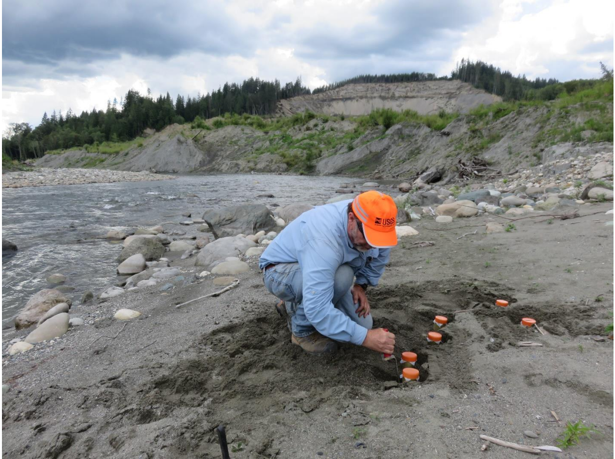
Figure S2. Soil-sampling method used to collect surface alluvium samples for geotechnical triaxial testing. The sample location is a newly formed river sand bar on the upstream end of the 2014 Oso landslide and thus representative of the surficial alluvium present in the floodplain prior to being overridden by the landslide.
