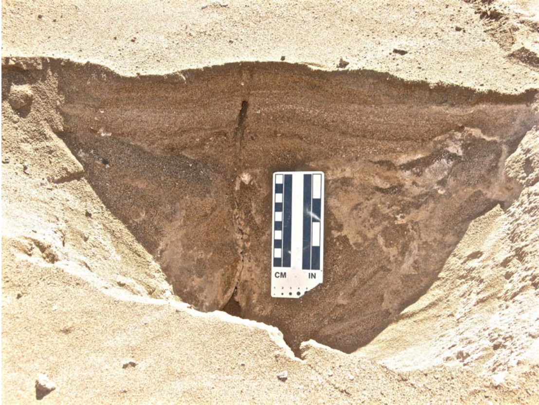
Figure DR9: Excavated crack profile showing that walls degrade near the surface. This photo is of a crack opening produced during the 2007 M_w 7.7 Tocopilla earthquake. Crack opening in the more competent material at the depth of the scale may better reflect the coseismic strain than the apparent crack opening in the looser sand. Loose eolian sand accumulated in an old surface crack depression has enhanced the new crack opening, which overlies a very fine crack in gypsum fill (lighter material where the scale is located).
