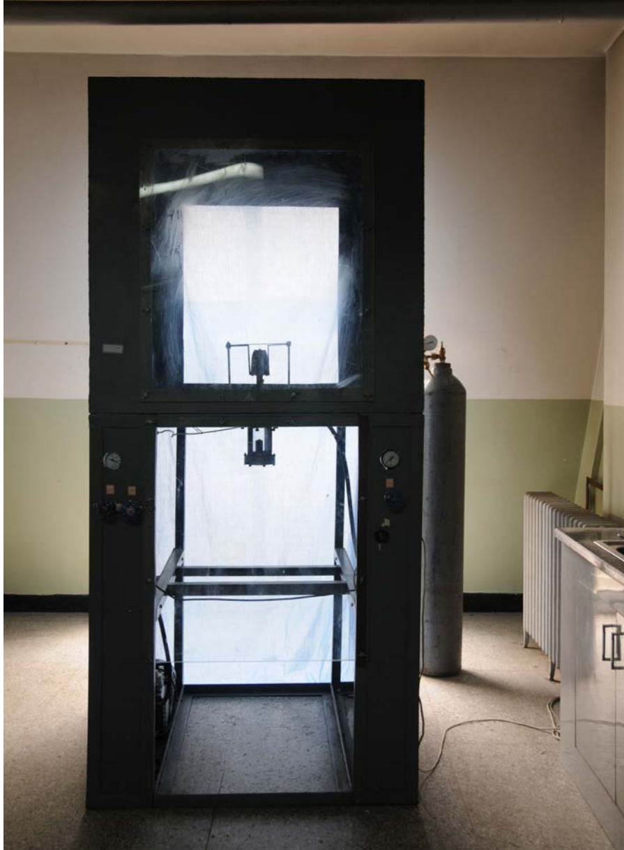
Figure DR1. Experimental apparatus for coal outbursts. A coal cylinder is inside the test cell.
