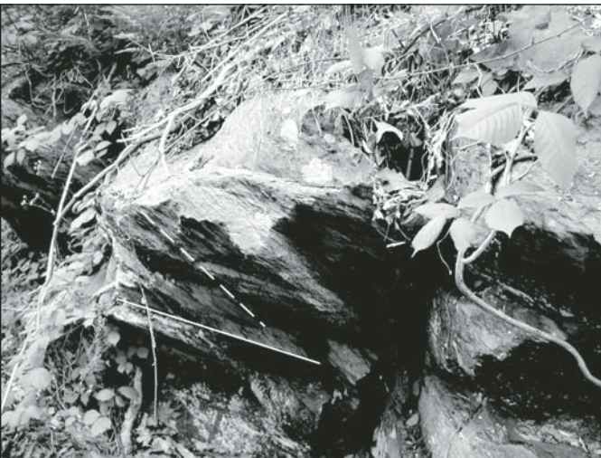
Figure 19. Cleavage (dashed line) in shale and siltstone dipping more steeply than bedding (solid line). Be careful of the plant with leaves of three...“let it be.”
